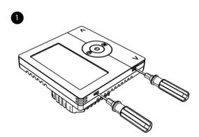
Remove the front cover by prying hooks with flat screwdriver at the bottom of the front panel
