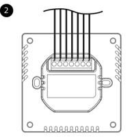
For the convenience of installation, the first step is to wire the volt-free wires, lowvoltage wires then high-voltage wires. Check the wires are property connected.
