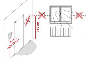
Devices must be mounted on clean, dry indoor place without direct airflow from a heating / cooling device, and not be exposed to dripping or splashing
